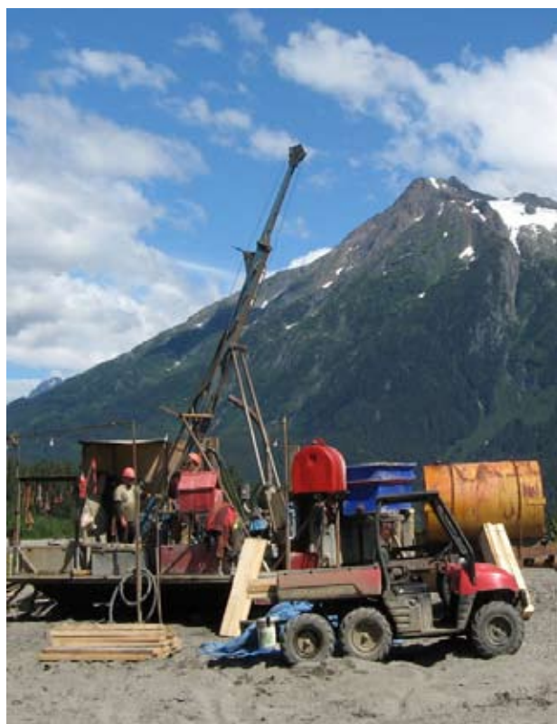
Infill drilling to depths of 600 m
