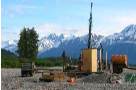
Diamond drill rig testing the C vein system
