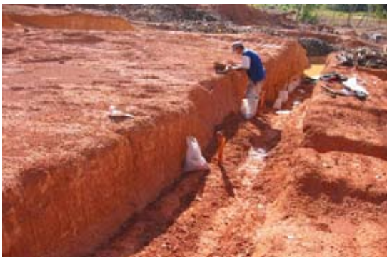
Channel sampling of gold mineralization in pork-knocker pits
